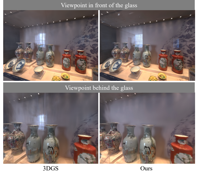
Fig. 2. Rendering comparison of 3DGS (left column) and our method (right column) from two viewpoints — in front of the glass (top row) and behind the glass (bottom row). Our method effectively disentangles reflection and transmission components: clear reflections occur solely on the glass’s front side; no reflections are visible from behind. By comparison, 3DGS fails to accurately model reflections on transparent glass, producing many floaters of “reflection ghost” far from the real surface.
